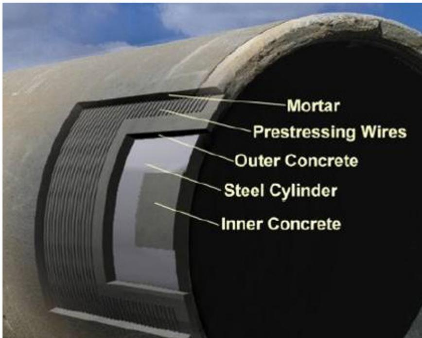
This cutaway diagram shows the components found in PCCP pipe.
