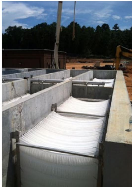
A close-up of the attached growth media—the media fabric sheets provide a means for the biology to physically attach.
