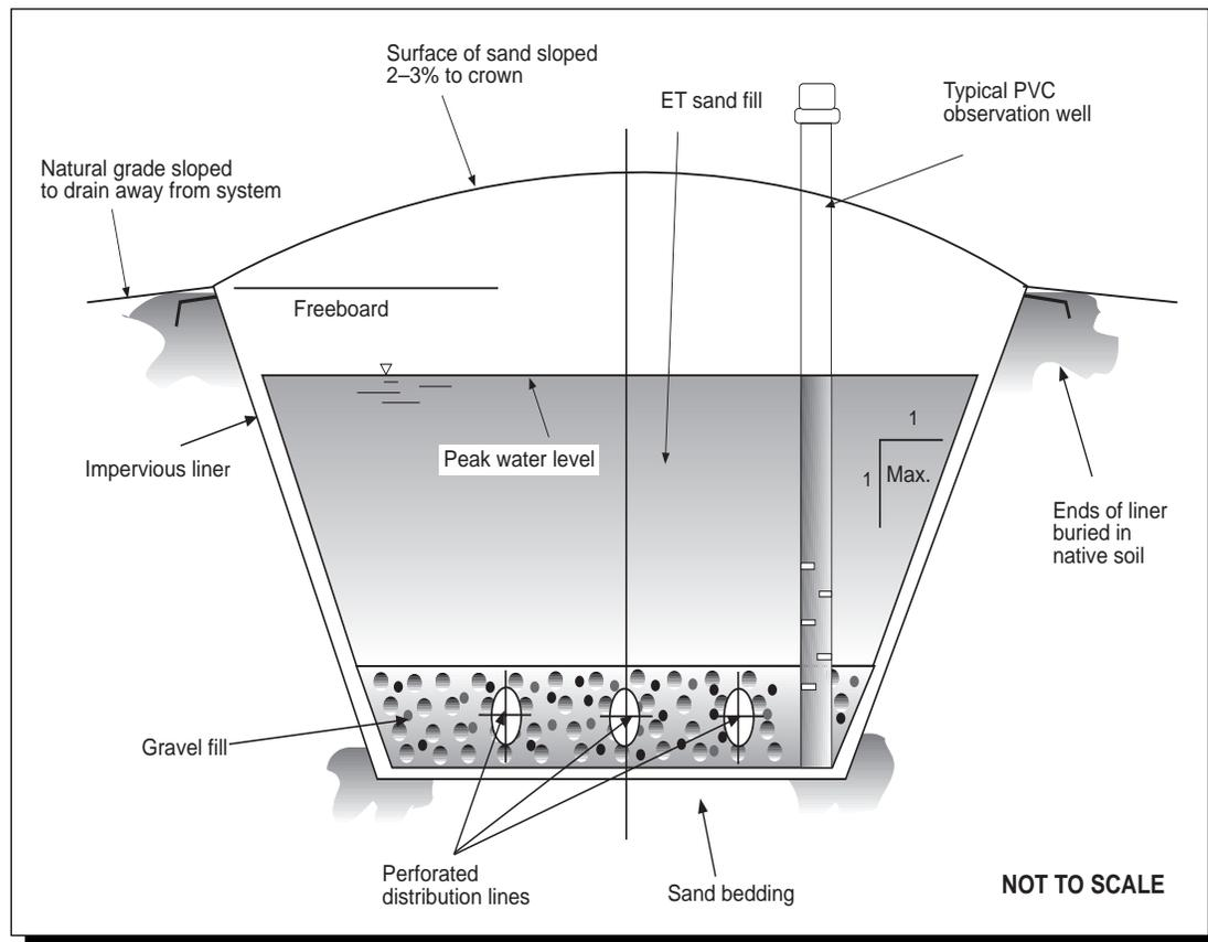
**Figure 1: Cross Section of a Typical Evapotranspiration Bed**
