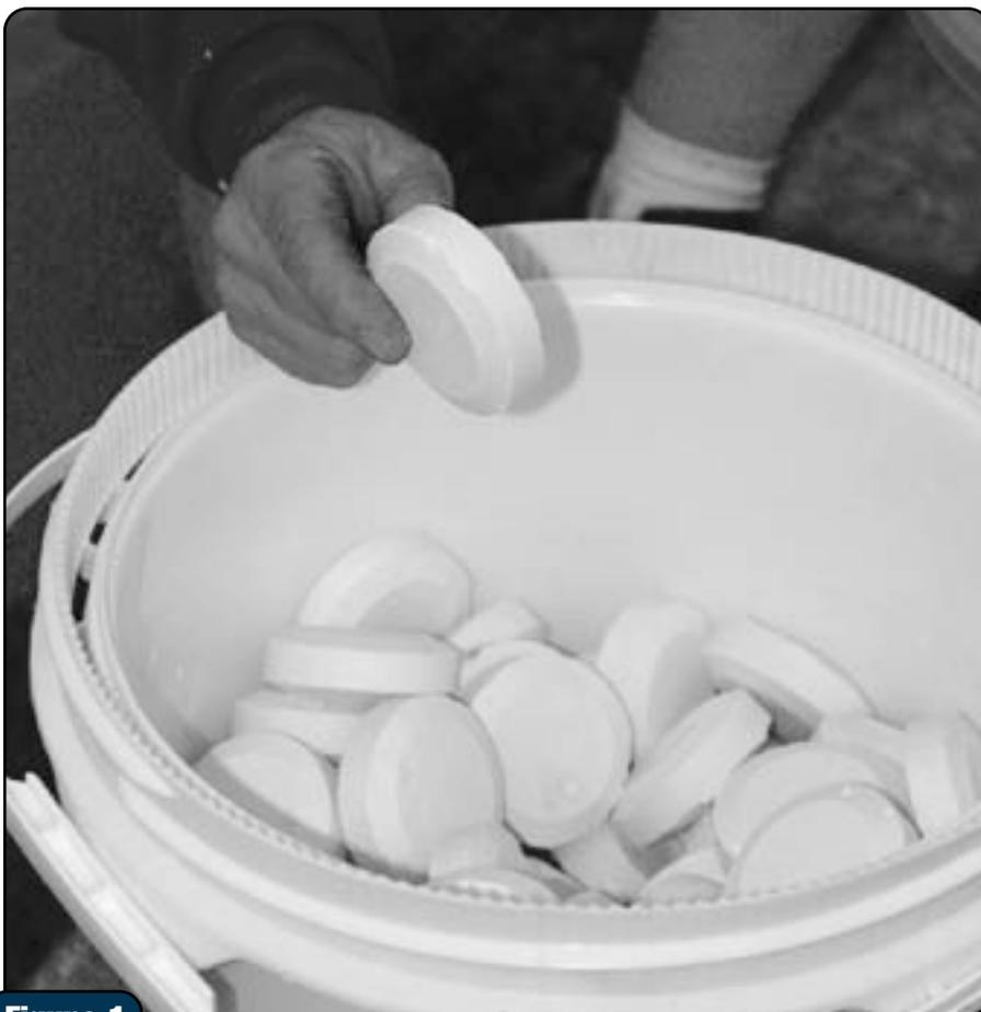
**Figure 1** Chlorine tablets (calcium hypochlorite) for use in tablet feeders. [Please note that operator should wear gloves when handling chlorine tablets.]
