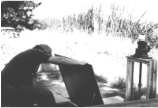
Marsh water levels at Arcata are checked using wet wells. (Photo by Deborah Carol.)
