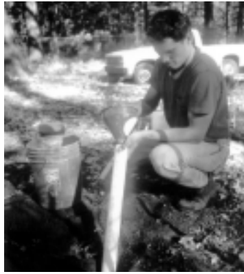
At the Paradise, CA, NODP site, students from California State University, Chico installed suction lysimeters to monitor groundwater contamination. Here, a student takes samples. (Photo by Stewart Oakley.)
