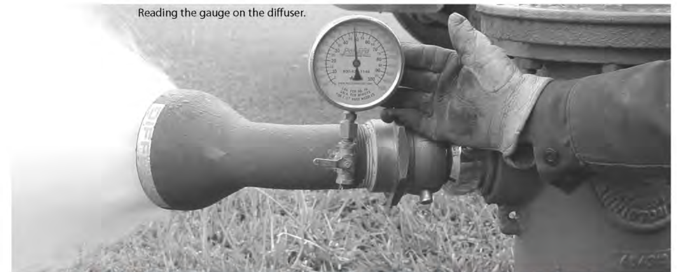
This pitot gauge is showing approximately 50 pounds per square inch (psi) of pressure or approximately 1,190 gallons per minute (gpm) of flow.
